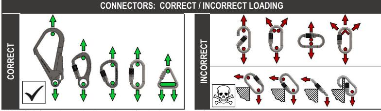
WARNING! Before each use a visual inspection and functional test must be performed by the user!
